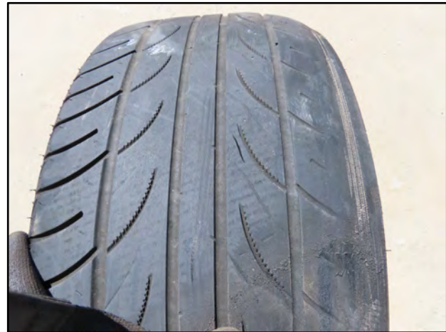
Figure 37. View of the left-rear tread package wear.
