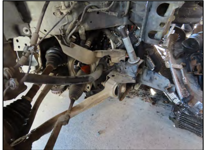
Figure 22. Displaced right-side suspension.
