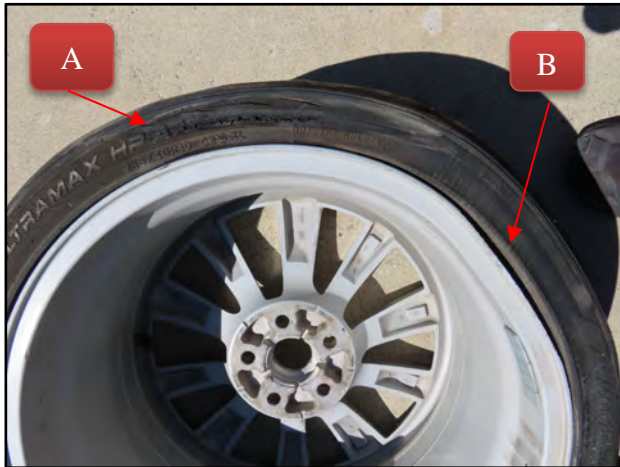
Figure 36. Inboard view of the left-rear tire and wheel damage.
