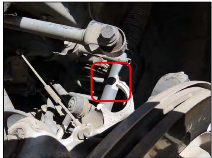
Figure 35. Fractured rear knuckle.
