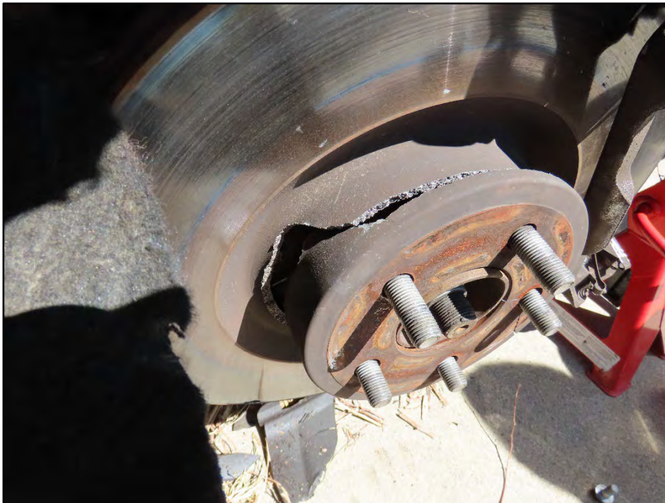
Figure 24. Fractured left-front brake rotor.
