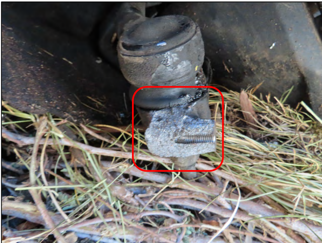
Figure 20. Fractured left steering knuckle.
