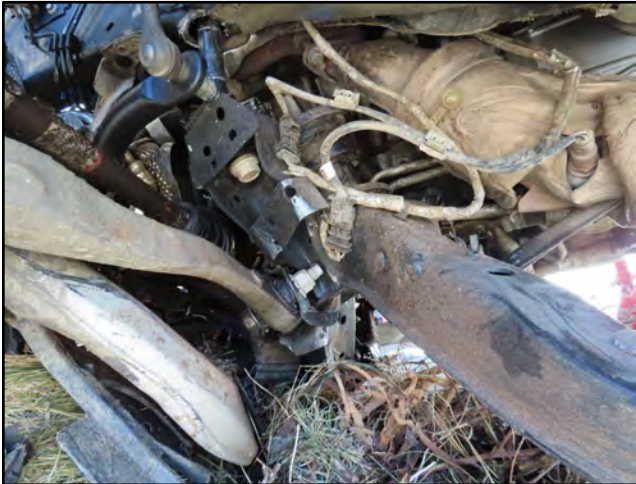
Figure 21. Displaced left-side suspension.
