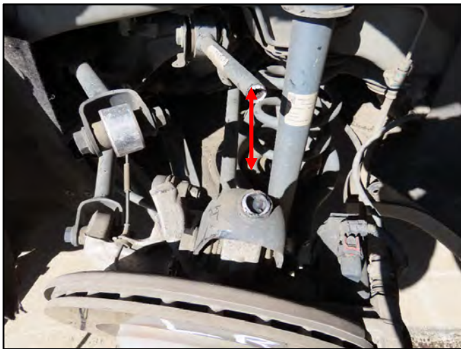
Figure 34. Fractured upper control arm.
